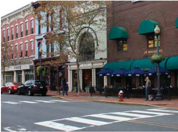
Curb Bump outs are simple extensions of the curb that calm traffic and reduce pedestrian crossing distance. They can be used to provide additional sidewalk width for outdoor dining etc (Red Bank, NJ - left) or they can be used as “flow through” planters for storm water management (right).
